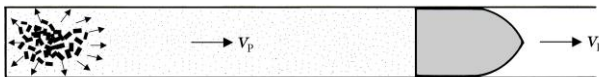
Fig. 8.3 At the moment of maximum pressure, the burning propellant is generating gasses at the same rate as the volume is increasing. The whole gas column thus has the same velocity as the projectile.
